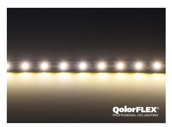
QolorFLEX LED Tape, Warm White, 12V Indoor (P/N 3528-12-WW-60-5-20-1) is an interior grade LED tape with a medium low output (300 lumens/metre) brightness and a warm 2700°K colour temperature. Each LED tape comes with wiring leads on both ends and durable 3M adhesive backing. It is available in full five metre reels and sample strips.
